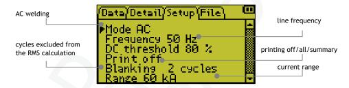
The **Mode** parameter determines the type of welding current to be measured, AC or DC.
