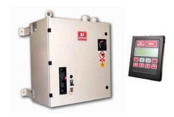
Control cabinet with door-mounted timer, up to 64 programs, constant current control and monitoring. Fitted into a sheet steel enclosure with circuit breaker, 24 VDC air valve power supply, appropriate line fusing, safety covers, and water-cooled MFDC Inverter Module. Optional hand-held pendant.
