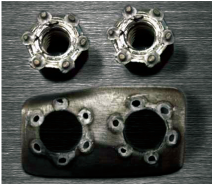
Fig. 5 — Overheated weld showing a large HAZ.
