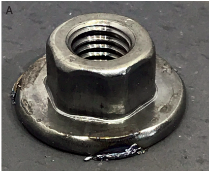
Fig. 5 — Overheated weld showing a large HAZ.
