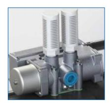
Calibrated during production, the valve never needs further adjustment. If anything happens to the electrical or mechanical components of the servo valve, end user maintenance staff simply disconnect three cables, loosen four bolts, remove the damaged servo valve and attach a pre-calibrated replacement valve, in stock at all times.
