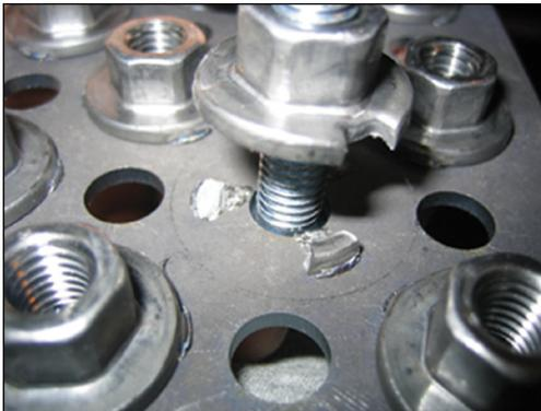
**Figure 2: M8 Nut welded to 2 mm boron**
